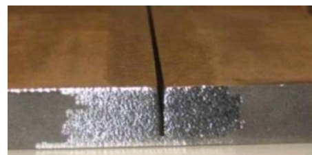
Fig. 4 1.5 mm groove machined down the center/middle of the plate
